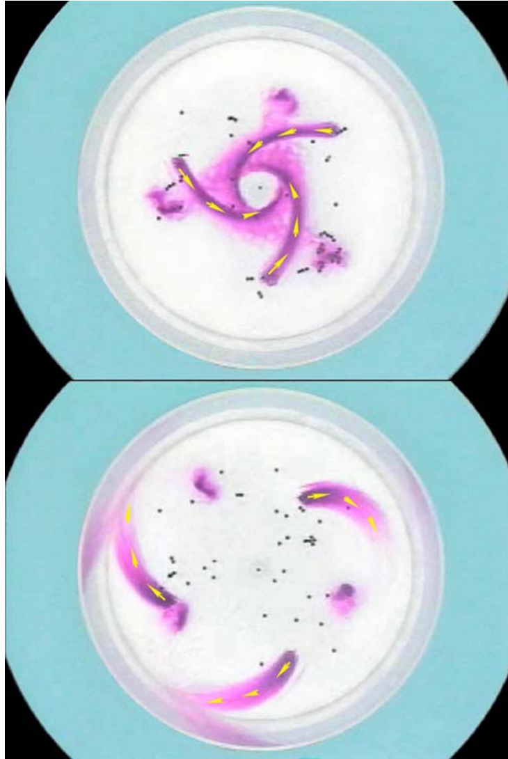
Figure 7.23: Ekman flow in a low pressure system (top) and a high pressure system (bottom) revealed by permanganate crystals on the bottom of a rotating tank. The black dots are floating on the free surface and mark out circular trajectories around the center of the tank directed anticlockwise (top) and clockwise (bottom).
