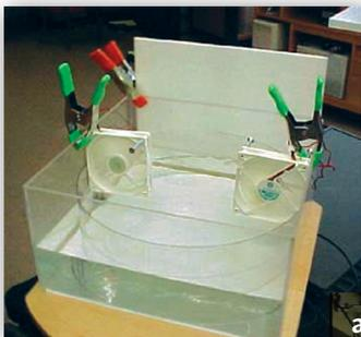
Figure 3. This photo shows the clear square tank sitting on a turntable. The computer fans are clamped to the sides. Also visible is an insert rendering a square tank circular. A white sheet acts as a back screen to visualize the flow in the vertical plane.
