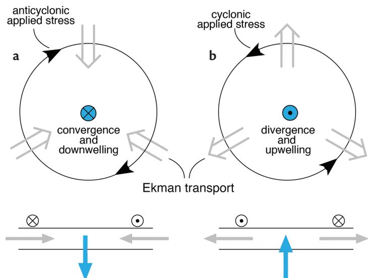
Figure 2. The Ekman transport is directed perpendicular to the applied stress (to the right if  $\Omega > 0$ , to the left if  $\Omega < 0$ ), driving (a) convergent flow if the stress is anticyclonic and (b) divergent flow if the stress is cyclonic. (The case  $\Omega > 0$ —appropriate to the northern hemisphere—is shown.)
